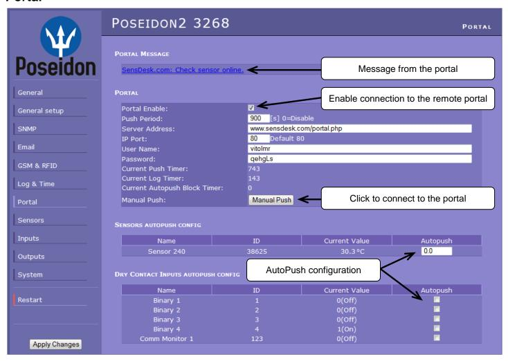
Configures the communication with the portal using the HWg-Push protocol. Poseidon2 is the active side and establishes the connection periodically and/or whenever a change in a sensor value exceeds the configured AutoPush value.
