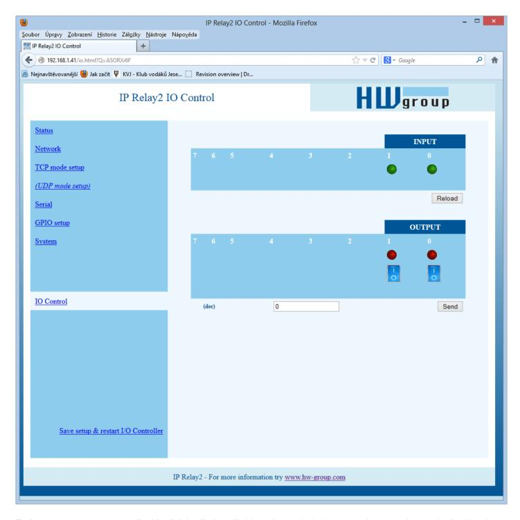
Relay outputs are controlled individually by clicking the switch icons, or by entering a decimal value and clicking Send.
