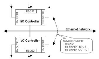
Virtual extension of the serial port + 8 inputs and 8 outputs over TCP/IP.
