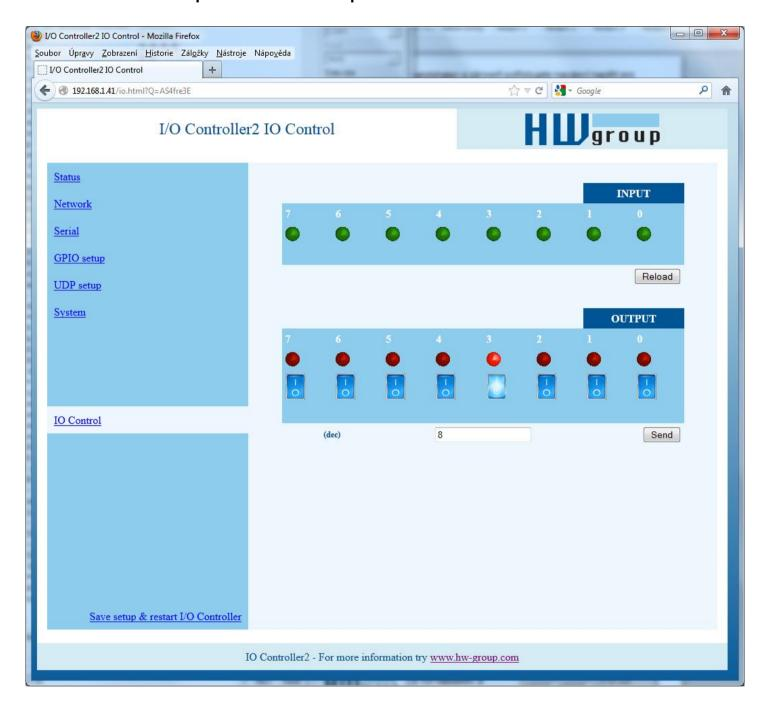
Outputs can be controlled either by entering a decimal value 0–255 corresponding to the output states, or by toggling the switches at the WWW page.
