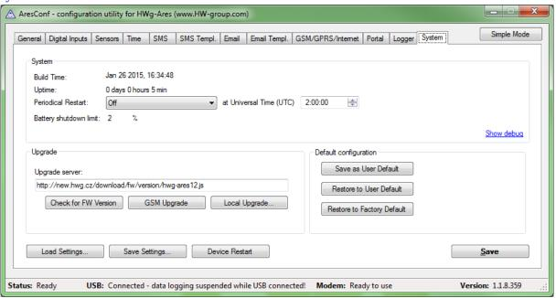
Use this tab to display and set system variables, upgrade firmware, and save or restore configuration.
