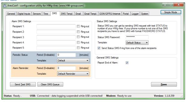
Use this tab to configure alarm text message (SMS) recipients. Each recipient phone number is also authorized to request information from Ares 12 by dialing the unit's phone number and to send SMS commands without a password (see Advanced settings).
