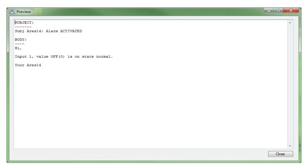
Use this tab to define the format of individual messages, e.g. to distinguish temperature alarm messages from humidity alarm messages or to define the contents of status and reminder messages.
