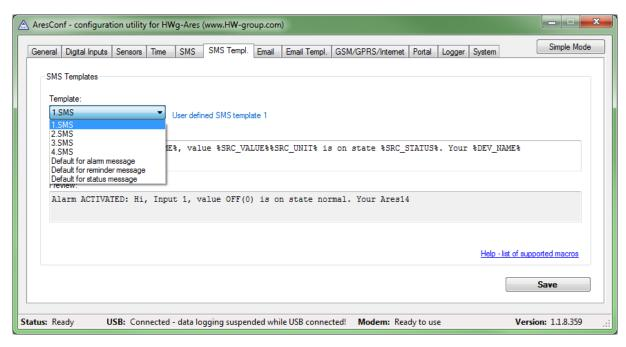
Use this tab to define the formats of individual messages, e.g. to distinguish temperature alarm messages from humidity alarm messages or to define the contents of status and reminder messages.
